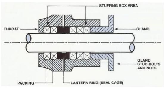
The importance of packing the pump correctly cannot be over-emphasized. Many packing failures are due to incorrect installation and maintenance of the packing. The following steps have been devised to ensure effective installation of compression packing on pumps.
